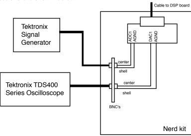
Note that since the BNC shell is tied to ground on the connected signal generator and scope, it is tied to the AGND pin on the DSP connector. Be sure not to reverse the polarity of this connection, as you may damage the DSP card electronics. If you have any questions about this, ask one of the teaching staff before making the connections.
