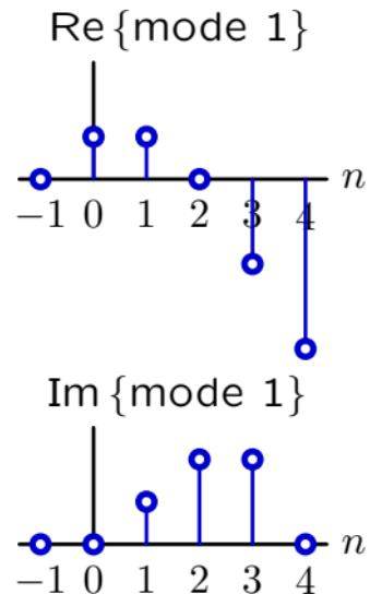
The output oscillates: poles off the real axis.
