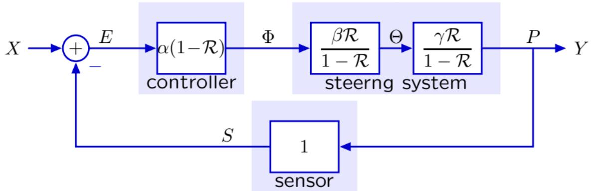
$$x[n] = 0 \rightarrow e[n] = -p[n] \rightarrow \phi[n] \propto (p[n] - p[n-1])$$
