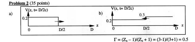
c) The Thevenin equivalent source at the end of the TEM line is twice the forward wave, or a 0.4 volt step function, delayed by D/c seconds. This charges the capacitor with  $\tau = RC = 4Z_o x$  D/8cZ<sub>o</sub> = D/2c (seconds). The voltage V(z=D) across the load rises instantly to <sup>3</sup>/<sub>4</sub> of 0.4 volts, since the C voltage is initially 0. Then it rises further exponentially ( $\tau = D/c$ ) to the open circuit value of 0.4 volts, which is:
