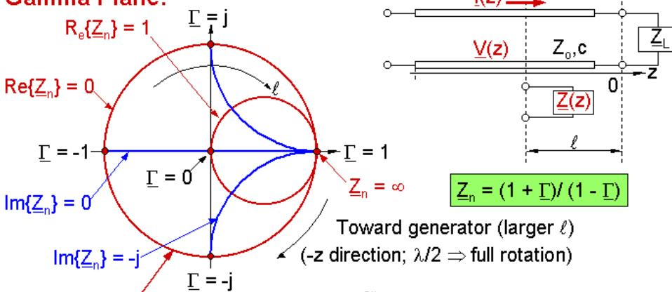
$$\underline{Z}_n = (1 + \underline{\Gamma}) / (1 - \underline{\Gamma})$$
