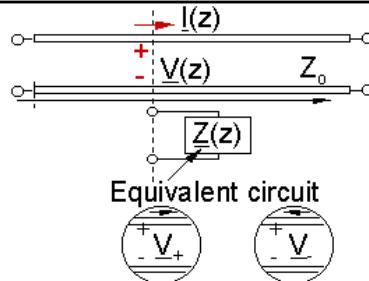
$$\underline{Z}(z) = \underline{V}(z)/\underline{I}(z) = \frac{Z_0 (\underline{V}_+ e^{-jkz} + \underline{V}_- e^{jkz})}{\underline{V}_+ e^{-jkz} - \underline{V}_- e^{jkz}} = Z_0 \frac{1 + \Gamma(z)}{1 - \Gamma(z)}$$
