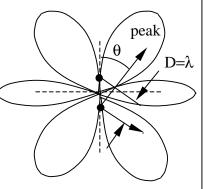
c) Maxima occur when the two signals add in phase, which occurs when  $\theta = \pm 90^{\circ}$ , and minima occur when the phase difference is maximum, which occurs when  $\theta = 0^{\circ}$  or  $180^{\circ}$ . The power at maximum is proportional to  $(1 + 1)^2$ , while at the minima it is proportional to the sum of the same two phasors, but at a phase offset of  $\lambda/4 \Rightarrow 90^{\circ}$ .  $1 - 1 - (1+1)^2 = 4$
