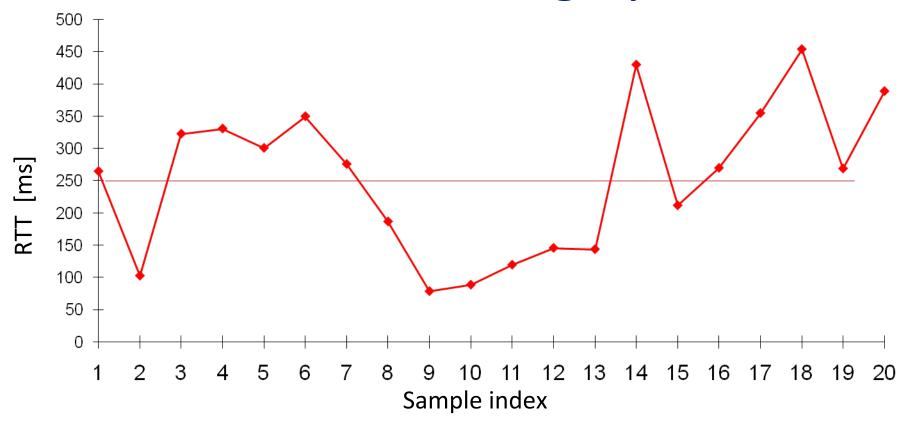
Example from a TCP connection over a wide-area wireless link Mean RTT = 0.25 seconds; Std deviation = 0.11 seconds!
