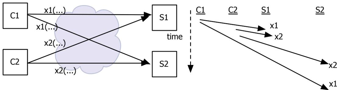
x1 is delayed from c1 → s2, arrives in different order on two replicas
