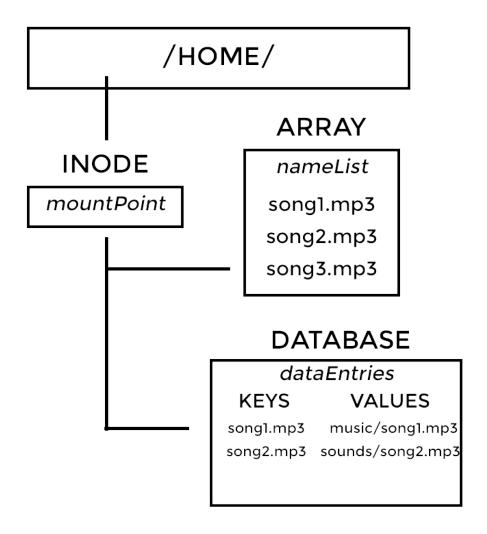
**FIG 2:** Visual Representation of the mountPoint inode and the two on-disk data structures, nameList and dataEntries. When the directory inode *mountPoint* is accessed initially, it calls upon nameList and dataEntries to create the DEP objects. The implementation is explored further in **3.2**
