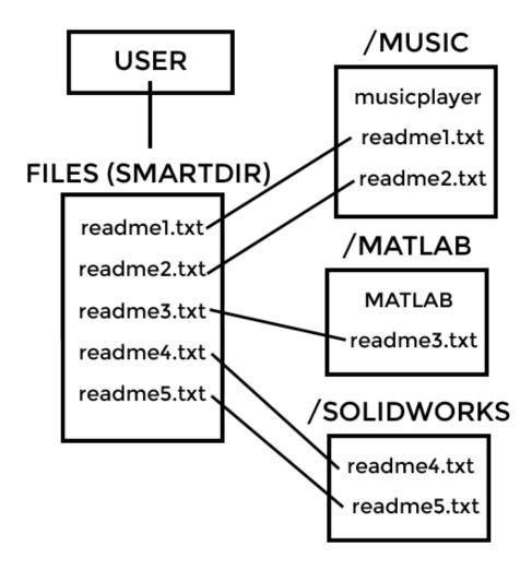
FIG 1. The user has created a SmartDir, with the expression "filename contains readme". The resulting SmartDir returns symbolic links to the files that meet the search criteria. The user can access the files from the SmartDir, rather than having to access each folder (/Music, /MATLAB, /SOLIDWORKS) individually.
