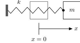
Extend the spring by a distance  $x_0$ ; this displacement is the amplitude. To see how it affects the period, make an approximation, which will be an example of throwing away information (the topic of **Part 3**). The approximation is to pretend that the pendulum moves with a constant speed  $v$ . Then the period is
