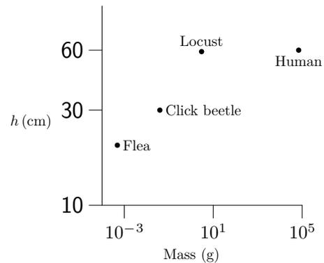
The height varies almost not at all when compared to variation in mass, so our result is roughly correct! The mass varies more than eight orders of magnitude (a factor of  $10^8$ ), yet the jump height varies only by a factor of 3. The predicted scaling of constant  $h$  ( $h \propto 1$ ) is surprisingly accurate.
