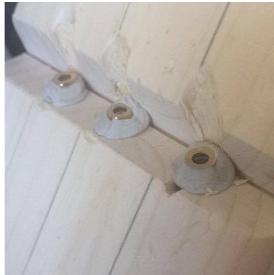
Figure 2B. The bottom row of laser diodes embedded in the laser harp
