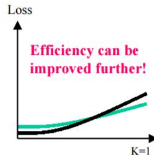
Figure 15. Comparison of loss in the power devices in a class AB amplifier versus a class D amplifier. The class D amplifier clearly wins!
