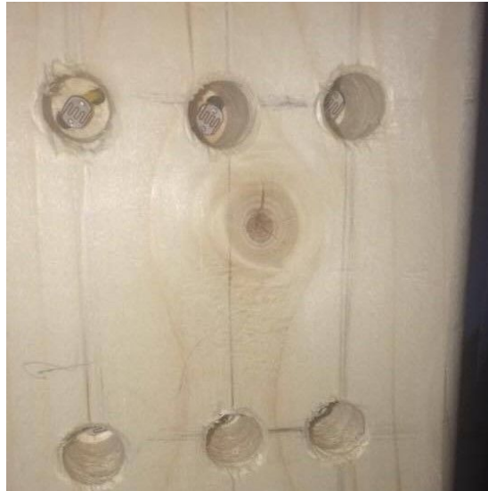
Figure 2A. The top row of photoresistors in the laser harp
