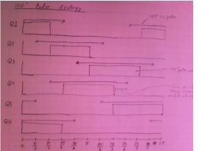
Motor is rotated by running currents through wire loops in a series of six states.
