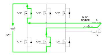
By applying a PWM wave to switch between these two configurations, we can control the level of current being supplied to the battery.
