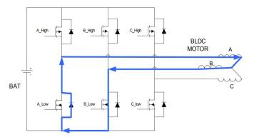
By switching between these two paths using a PWM signal, we can control the speed of the motor.
