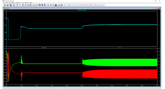
Fig. 14. Step response test with real-simulated components, from 2 A to 5 A Buck-boost L = 10 \mu\text{H} , C = 2000 \mu\text{F} . K_p = 1 , R_i = 10 \text{ k}\Omega , C_i = 330 \text{ nF}
