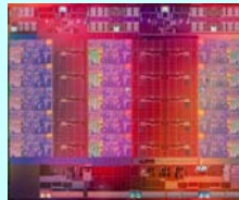
Intel Cascade Lake 2018 - 22 Cores >>7 Billion 14nm
