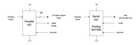
An example of a serial ADC is the Analog Devices AD7485, a 14 bit AD converter with serial output. The AD7485 uses a system clock, MCLK, provided by the user. To start the AD conversion, assert CONVST\_bar (bar = line above CONVST, an active low signal) low. SCO is system clock out which you can ignore for this exercise.
