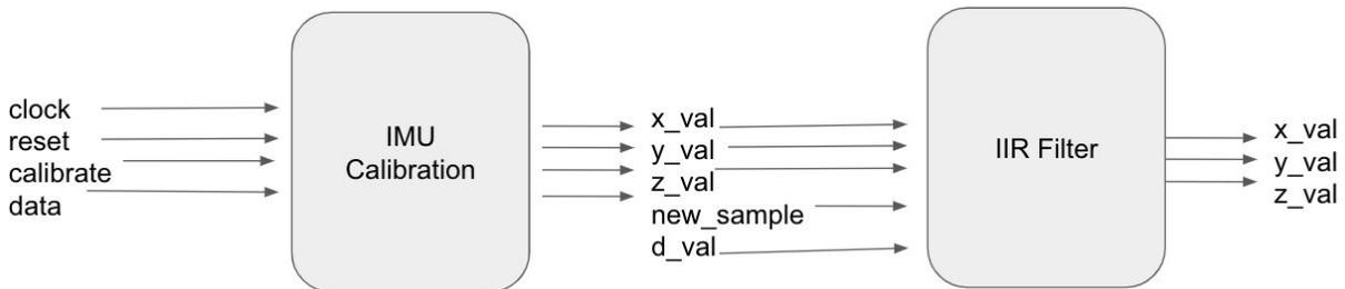
To test this module, we could create a test bench with dummy signals to make sure the IMU is reading in data in the proper cycles (i.e., waiting for data at appropriate times, reading at appropriate times).
