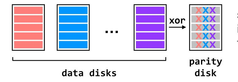
sector i of the parity disk is the xor of sector i from all data disks + can recover from single-disk failure
