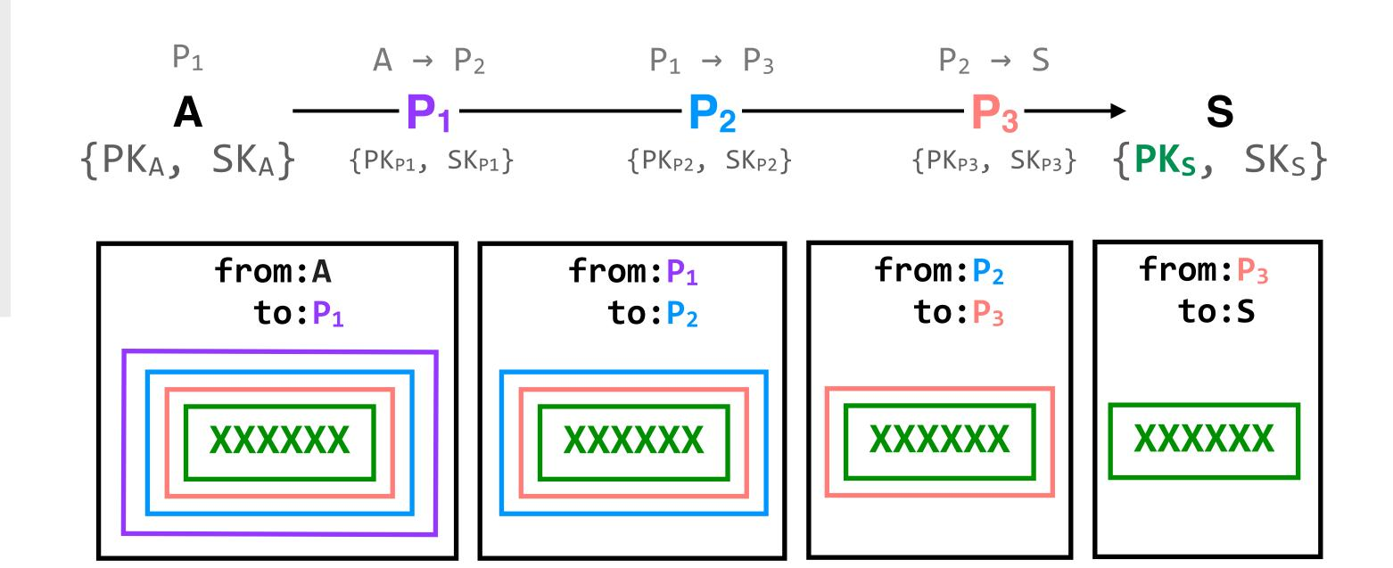
onion routing adds layers of encryption that nodes on the path can strip off as the packet traverses the network
