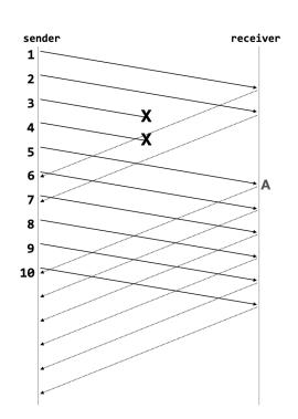
**A.** When the receiver sends an ACK in response to packet 5 (indicated on the diagram by the letter A), what will its sequence number be?
