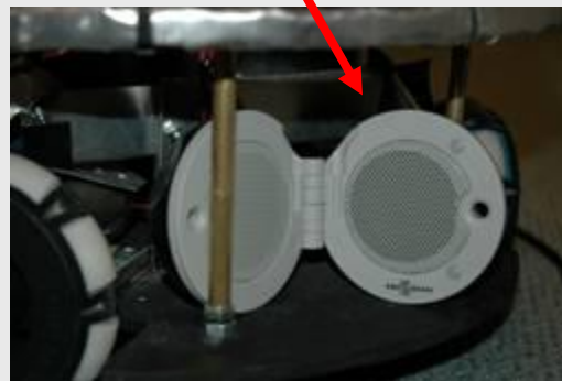
Speakers (played R2D2 sounds. Useful for debugging state changes).
