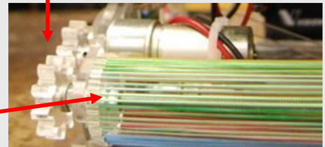
Geared drive – Note the wide gear, bearing length, and tolerance
