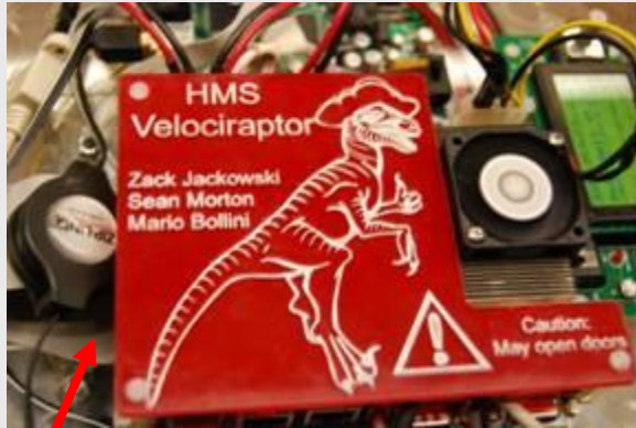
Computer Cover – Prevent Short Circuits!
