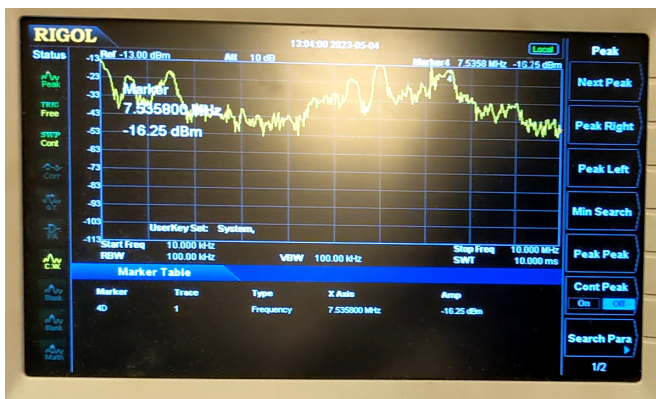
Fig. 4. RF preamp testing on Rigol spectrum analyzer
