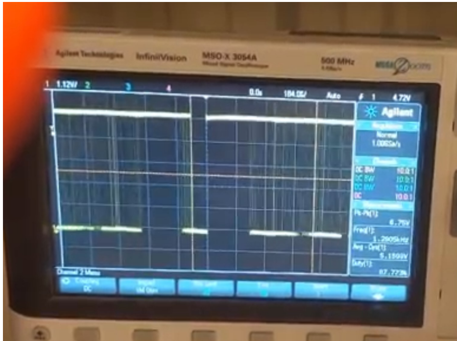
Fig. 8 Pitch circuit signal when the musician's hand is far away
