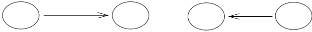
Figure 6: A two cell configuration where both pads are in range of their respective base stations and also in range of each other. The base stations are sending data to their respective pads, and each stream is generating data at a rate of 64 packets per second and using UDP for transport.
