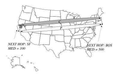
Figure 3-7: MED's are useful in many situations, e.g., if *C* is a transit customer of *P*, to ensure that crosscountry packets to *C* traverse *P*'s (rather than *C*'s wide-area network). However, if *C* and *P* are in a peering relationship, MED may (and often will) be ignored. In this example, the MED for  $D_SF$  is set to 100 at the SF exchange point, and 500 in Boston, so *P* can do the right thing if it wants to.
