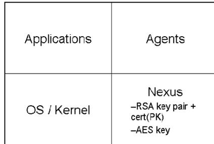
Figure 1: Palladium model. The keys shown here in the nexus are actually in a separate chip called the SSC.
