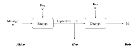
Figure 1: Sending a message over the network.
