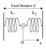
(c) If I turn the device on end, so that the springs hang vertical, what is the effect on the position of the stable configuration and on the motion of the mass when displaced? Assume the springs themselves have negligible mass.
