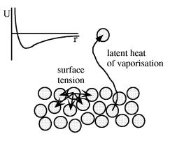
stituent atoms or molecules of a liquid interact with one another via intermolecular forces: a schematic diagram of the relevant potential energy is shown in the diagram. An atom at the surface is in an asymmetric position, and a net force will act to pull it in towards the body of the liquid: it has a higher potential energy than an atom in the interior of the liquid.
