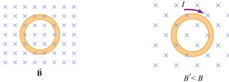
Figure 10.1.3 Inducing emf by varying the magnetic field strength
