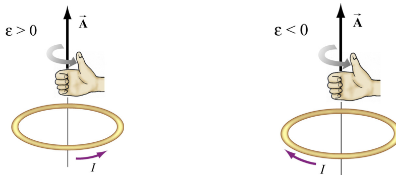
Figure 10.1.6 Determination of the direction of induced current by the right-hand rule
