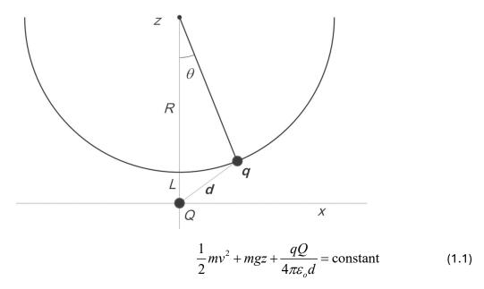
A charge q is located at (x, z) in the presence of a stationary charge of the same sign Q sitting at the origin. The charge q swings on a pendulum of radius R under gravity. When the charge q is at the bottom its swing it is a distance L just above the charge Q.
