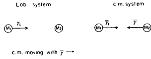
Fig. 12. The lab and center-of-mass systems for two particles colliding with different masses.
