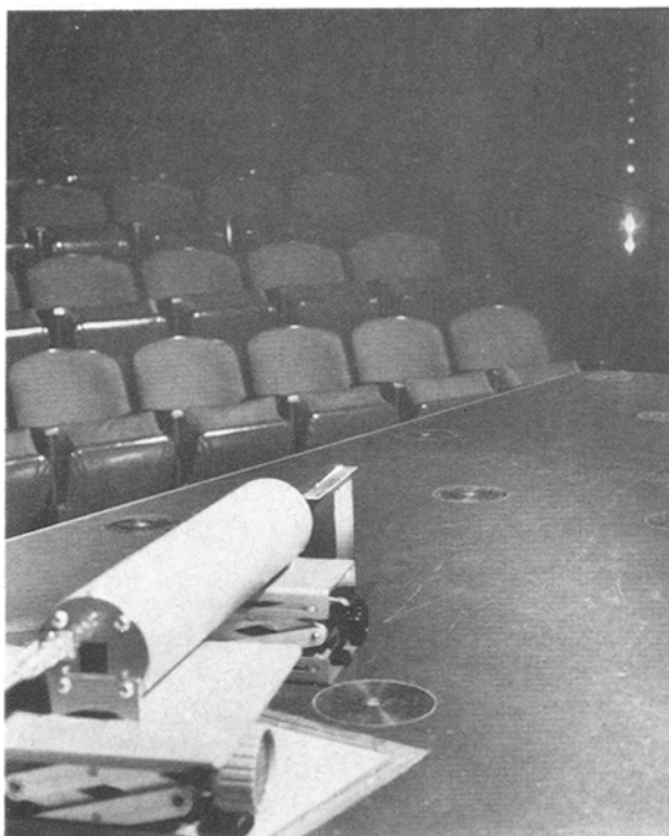
FIG. 1. Arrangement of the apparatus. The laser in the foreground shines on the rulings of a ruler, producing the diffraction pattern on the far wall.
