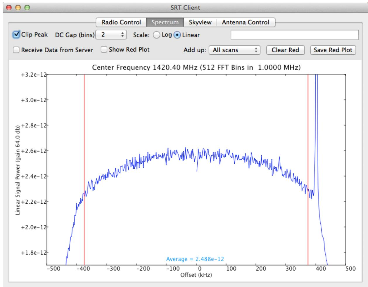
To correct for this pre-filter roll-off, I measured carefully the FFT signal (with an integration time of about 1000 s) from a white source (the Sun) and folded the upper and lower sideband signals on top of each other. Then I fit the average for bin numbers,  $\leq 192$ . The fit was very good and gave the normalised result
