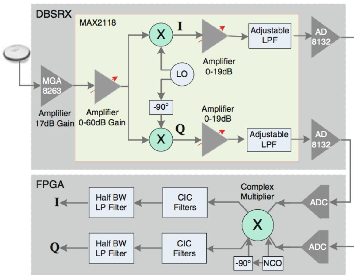
The figure is for a DBRSX daughterboard (with a MAX2118) but I think is otherwise the same as ours. The output from the Half BW filters is sent by GHz Ethernet UDP as a stream of complex integers (16-bit signed real and imaginary parts) to the computer in 26-630 at the sample rate selected by the server software on the computer. Usually that is 1.00 or 1.25 MHz, but can be as high as 5.0 MHz—which requires a 160 Mb/s Ethernet data rate.
