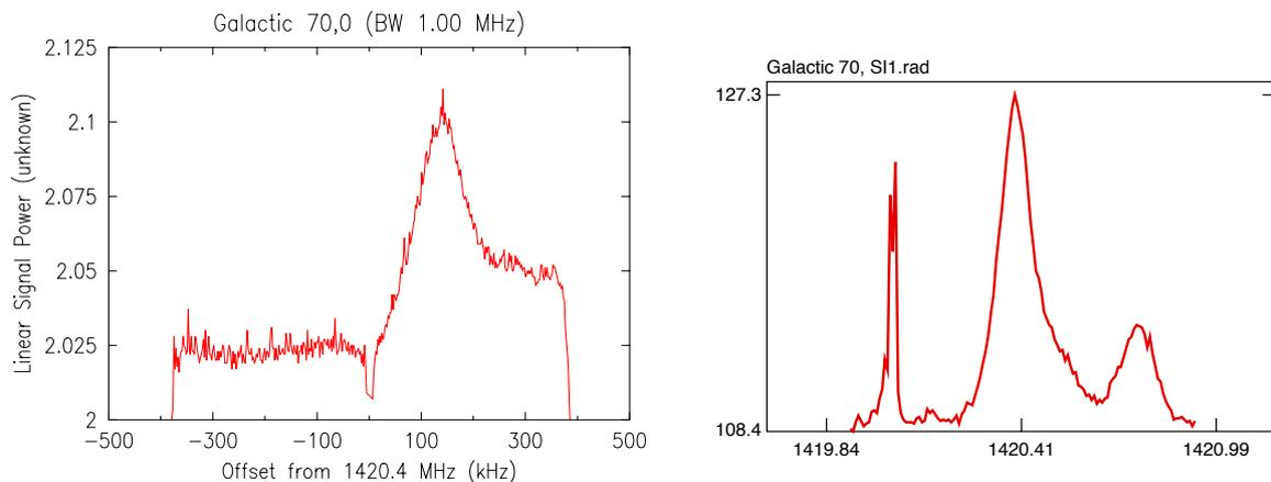
The peaks look similar. The SRT data have an interference peak at about 1420 and the NSRT data notch at zero offset is, I think, the result of an imbalance in the USRP2. It can be either a notch or a peak depending on the receiver gain and is usually about two FFT bins wide.
