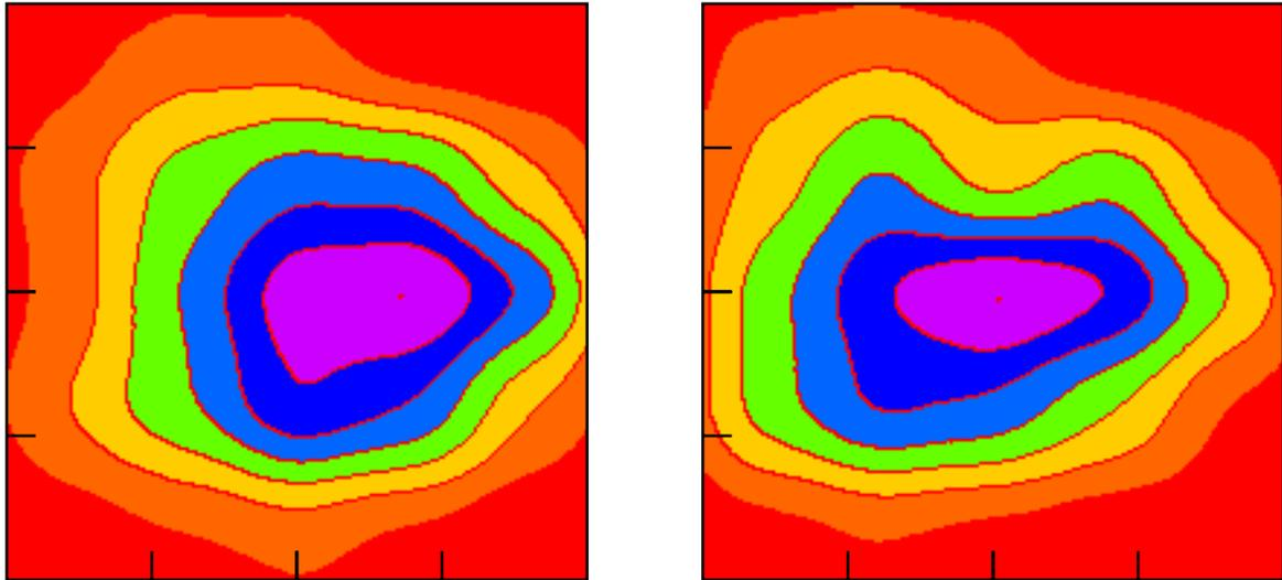
Two days later I repeated the Sun npoint scan and got the result above on the right. So the pointing calibration seems to be good.
