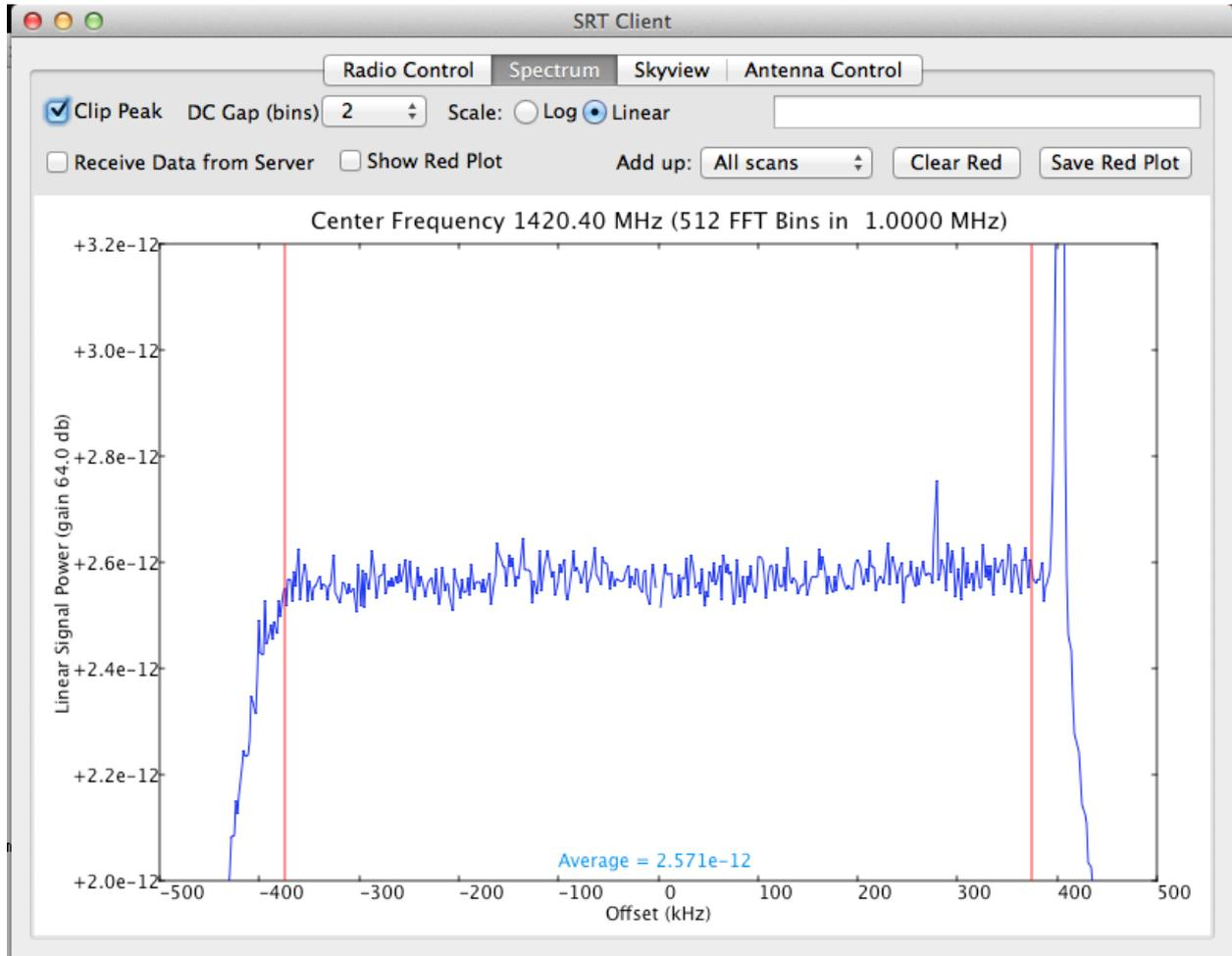
I did this for sample rates of 1.00 MHz and 2.00 MHz. I wrote the software in `bernieClientG.py` to restrict sample rates to 11 values from 416 kHz to 5.00 MHz that gave even decimation values with the 100 MHz DSP. It turned out that the 1.00 MHz corrections worked very well for sample rates 1.25 MHz and below as well as 2.5 MHz and above. The 2.00 MHz correction had more curvature and worked well for 1.5152 MHz and 2.00 MHz. The equation for it was
