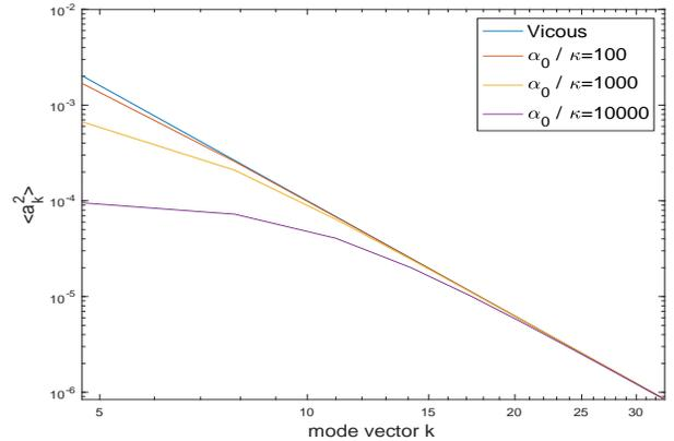
**Figure 2:** Mode amplitude variance with mode vector  $k$ . In this plot, we only look at the power-law between mode vector  $k$  and mode amplitude with tuning the ratio of the shear modulus to bending capacity and thus, other parameters irrelevant are arbitrarily chosen. Therefore, the unit of  $y$ -axis is also arbitrary unit.
