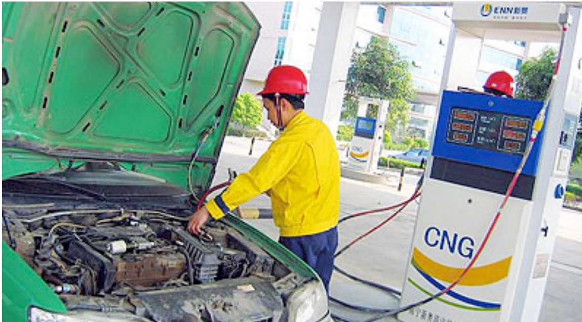
Figure 3: Filling Taxi Gas Tank with Compressed Biogas
