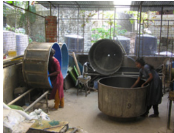
Figure 2: Fabrication of biodigesters with ferro cement
