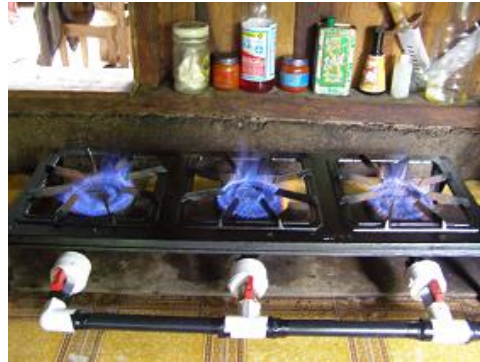
Cooking stove powered by methane
