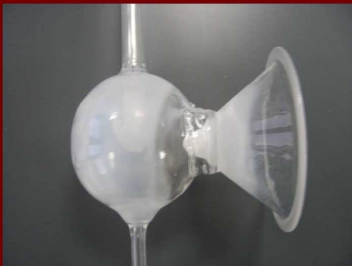
A cone, the tip of which is pierced with a 75 \mu\text{m} hole has been inserted in the reactor (made in France)
