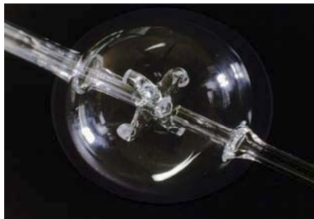
Jet stirred reactor
