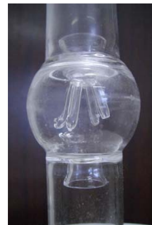
Jet stirred reactor
