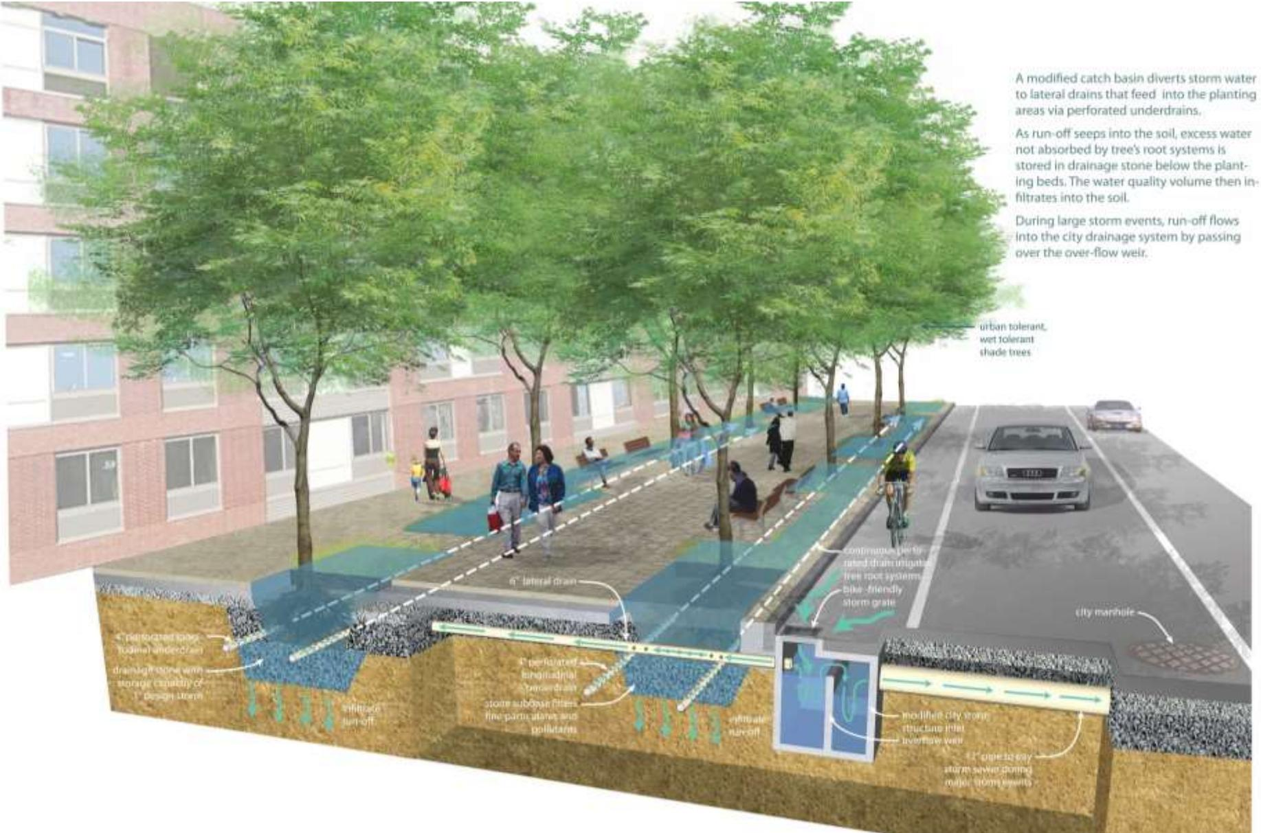
A modified catch basin diverts storm water to lateral drains that feed into the planting areas via perforated underdrains.
