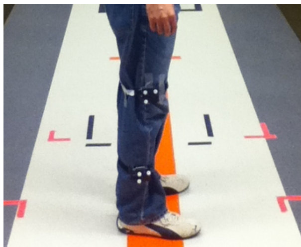
Fig. 2: IMU placement and reflective marker locations.
