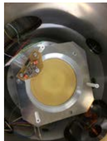
Figure 1. A prototype 10-cm diameter, 2.5-mm thick, single-strip silicon lithium detector mounted in a test chamber for calibration. (Photo: Kerstin Perez).
