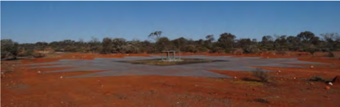
The EDGES antenna and ground screen deployed in the Western Australian desert, near the Murchison Widefield Array. The large mesh ground screen is shaped to minimize reflections from the transition from mesh to soil, and to maintain the required exquisitely smooth spectral response of the instrument.
