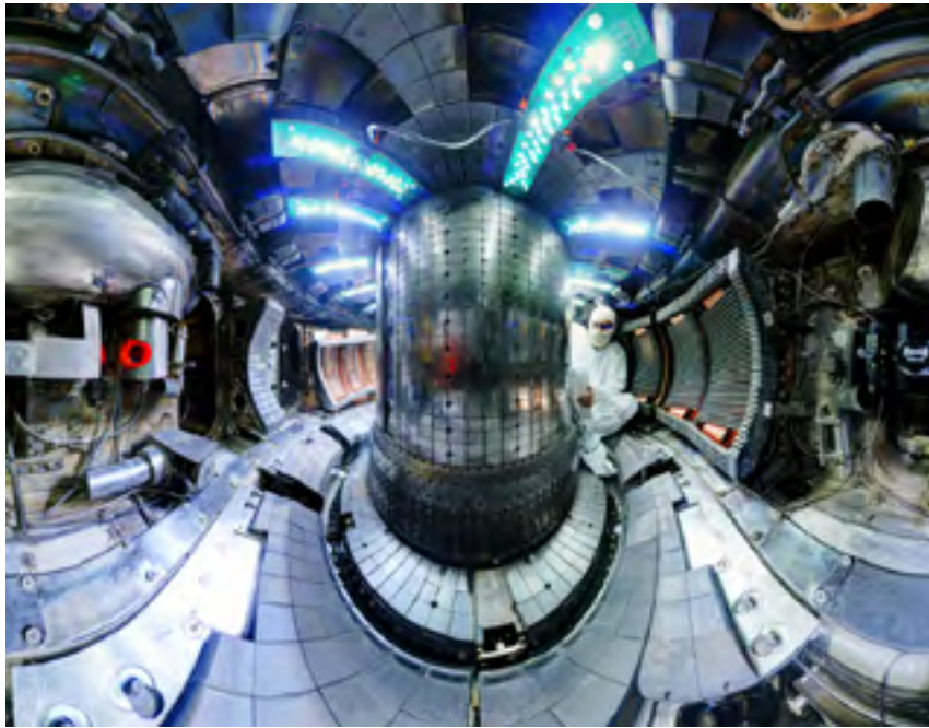
Figure 1. Mercator projection of the interior of the Alcator C-Mod tokamak, which broke the record for plasma pressure in a fusion device in September 2016 during the program's final experimental campaign.
