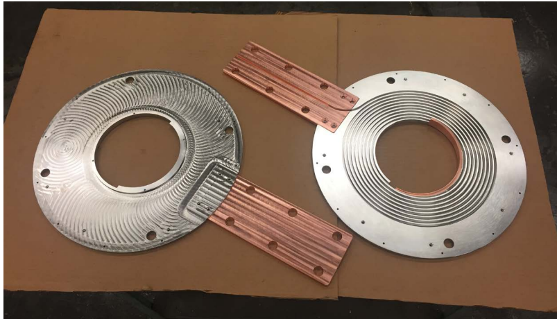
The two halves of a pancake coil fixture for testing new superconducting wire for the SPARC project at the Plasma Science and Fusion Center. Credit: Andrew Gallant.
