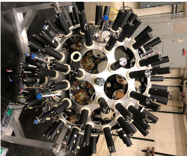
The NuDot detector consists of 140 2-inch photo-multiplier tubes (PMTs) and 72 8-inch PMTs mounted on an aluminum sphere, viewing the inside of the sphere. The 8-inch PMTs in the upper half and along the equator are yet to be mounted in this photo.
