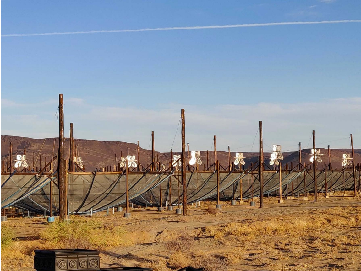
Dishes of the radio telescope Hydrogen Epoch of Reionization Array (HERA) that act in concert to observe intergalactic matter in the early universe. MIT Kavli Institute leads commissioning of the wide-band instrument feeds seen at each dish's focus.
