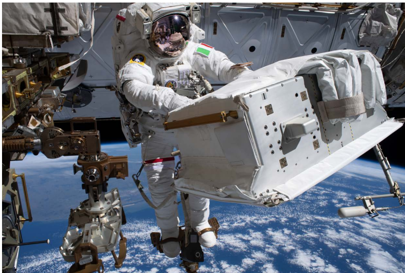
European Space Agency astronaut Luca Parmitano with the Upgraded Thermal Tracker Pump System (UTTPS), while on an Extra Vehicular Activity to mount the UTTPS on the Alpha Magnetic Spectrometer on the International Space Station.
