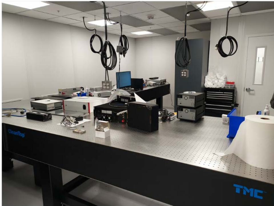
The new clean room in 24-035 built to house both low-power and high-power lasers for developing precision laser spectroscopy techniques to study radioactive molecules.
