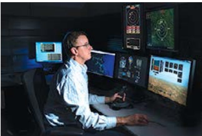
Figure 11. Lincoln Laboratory's Ground-Based Sense and Avoid system, operational at 12 military installations, provides maneuvering guidance to unmanned aircraft system operators to help them avoid nearby aircraft.
