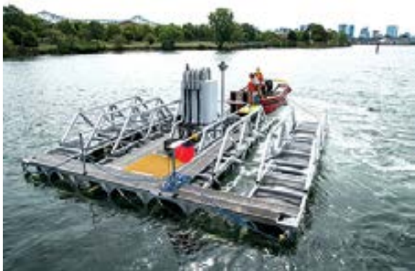
Figure 3. Researchers deployed a technology demonstrator of an undersea mapping sparse sonar array. The array is a novel surface-based, distributed multi-input multi-output sparse aperture sonar to support deep ocean floor mapping with a resolution two orders of magnitude higher than is currently achievable.
