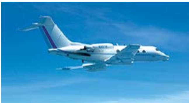
Figure 7. The Airborne Seeker Test Bed is a customized aircraft used in flight testing radio-frequency and infrared sensors. To carry these sensors, the aircraft is modified with wing pylons, a nose radome, forward chin-pods, and computer and instrumentation racks in the interior.
