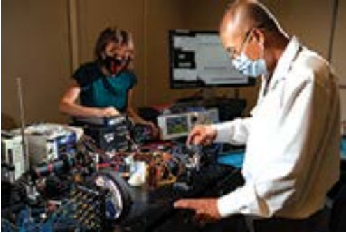
Figure 10. Staff are developing a near-infrared spectroscopy system that leverages our unique Geiger-mode avalanche photodiodes to improve measurements of brain activity. This project is a collaboration with Massachusetts General Hospital and is funded by the National Institutes of Health.
