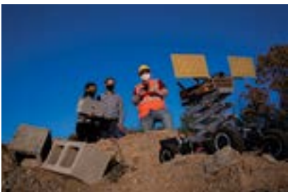
Figure 9. A radar system integrated on an unmanned ground vehicle can detect disaster survivors trapped under rubble. The radar extracts a breathing rate and wirelessly transmits the data and the location to rescue teams. Future work will focus on unmanned air vehicle integration.
