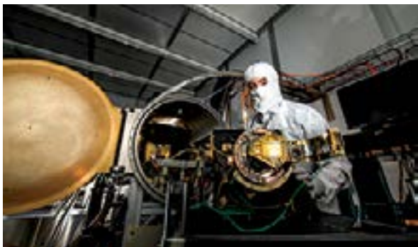
Figure 12. The sensor assembly for the Situational Awareness Camera Hosted Instrument is being placed in a thermal-vacuum chamber by a technical staff member in the Structural and Thermal-Fluids Engineering Group to replicate the environmental conditions of space where the instrument must operate.
