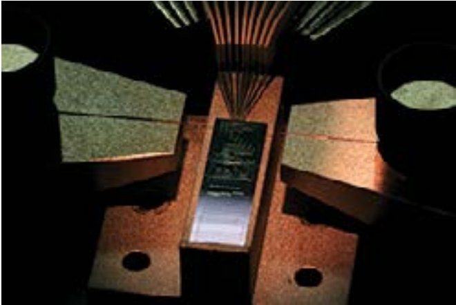
Figure 4. Photonic integrated circuit (PIC) optical matched filters achieved excellent filter extinction (>45 dB) and highly Gaussian lineshape. Coupled with advanced digital signal processing, PIC technology will dramatically reduce the size, weight, power, and cost of future lasercom terminals.
