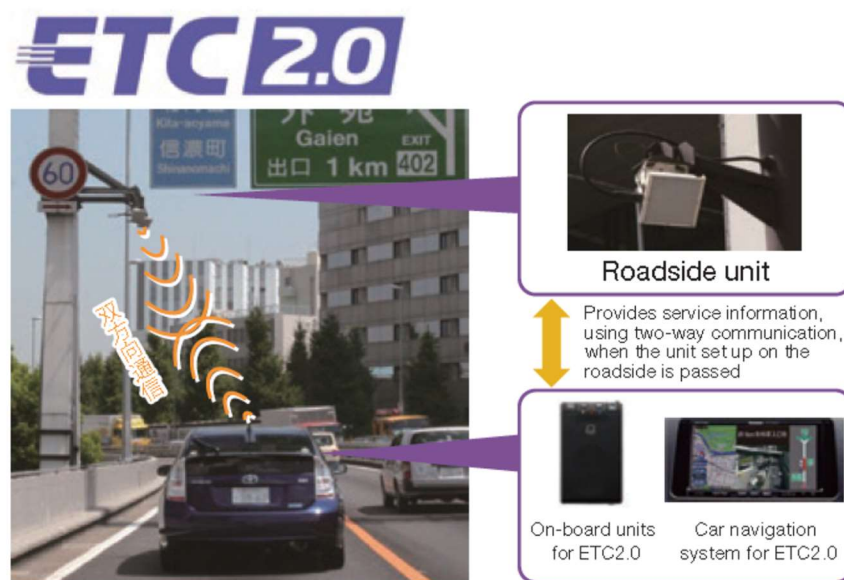
Figure 2.13: Electronic Toll Collection 2.0 (Source: White Paper on Land, Infrastructure, Transport and Tourism in Japan, 2015)
