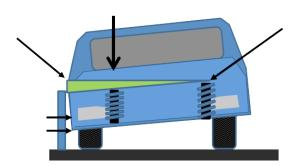
Initially, the meter stick is placed near the fender on the passenger side (which is the left side in the figure above). This was simply a convenient place to make the measurement of downward movement. In fact, we wanted to know the compression of the suspension spring which was substantially inboard of the fender.
