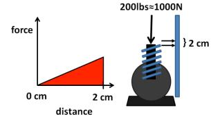
This is one interpretation of the answer to the question "How much energy does it take to compress the suspension spring?" We measured and calculated how much energy must be added from
