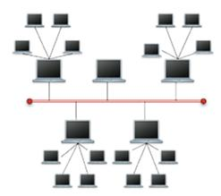
Star-Bus: The star bus topology is combined with the linear bus in large networks. In such cases the linear bus provides a backbone that connects multiple stars.
