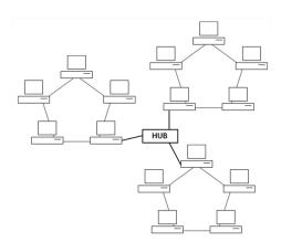
Star Ring: The Star Ring is a combination of ring and star topologies. The hubs in a star ring are connected in a star pattern by the main hub.
